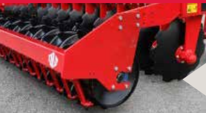
Soil deflector disc set right set of 2 adjustable side-discs. The first disc keeps the soil inside the working width. The second disc guides the soil to fill the furrow.
