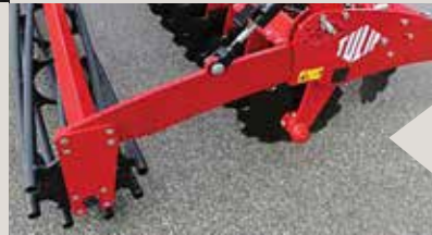
Hydraulic roller adjustment two cylinders, which make it possible to adjust the roller by using the tractor hydraulics.
