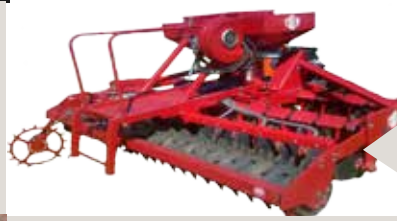
Hydraulic roller adjustment two cylinders, which make it possible to adjust the roller by using the tractor hydraulics.
