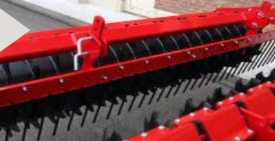
is mounted behind the last row of discs and assures an improved coverage of crop residue. The height and angle are adjustable.
