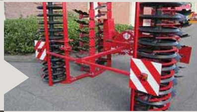
Soil deflector plate right a side plate which keeps the soil stream inside the working width.
