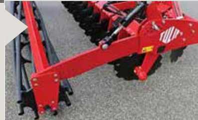
Hydraulic roller adjustment two cylinders, which make it possible to adjust the roller by using the tractor hydraulics.
