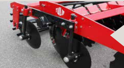
Straw harrow is mounted behind the last row of discs and assures an improved coverage of crop residue. The height and angle are adjustable.
