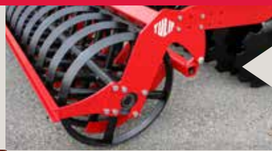
Soil deflector plate right a side plate which keeps the soil stream inside the working width.
