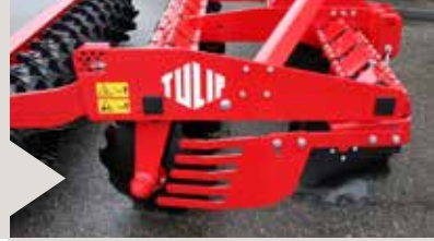
Soil deflector plate right a side plate which keeps the soil stream inside the working width.
