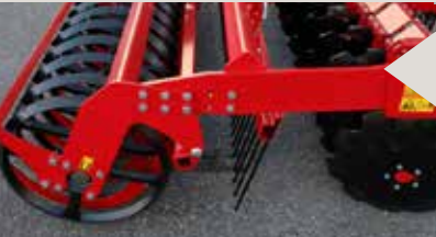
Soil deflector disc set right set of 2 adjustable side-discs. The first disc keeps the soil inside the working width. The second disc guides the soil into the furrow.
